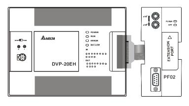
Once DVPPF02-H2 is connected to DVP-EH2 through the connection port, DVP-EH2 will be able to read or write the CR data in DVPPF02-H2 by using DFROM/DTO instruction. The data transmission between DVPPF02-H2 and PROFIBUS DP master is done through PROFIBUS DP bus.
