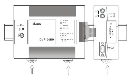
2.5 Connecting to PROFIBUS DP Connection Port Insert the PROFIBUS DP bus connector into the PROFIBUS DP connection port on DVPPF02-H2. Screw it tight to ensure DVPPF02-H2 and the PROFIBUS DP bus are properly connected.
