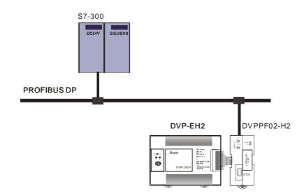
2. Set the address of DVPPF02-H2 to "11" (decimal). See "21.3.1 Address Switch" section for how to set up the address.
