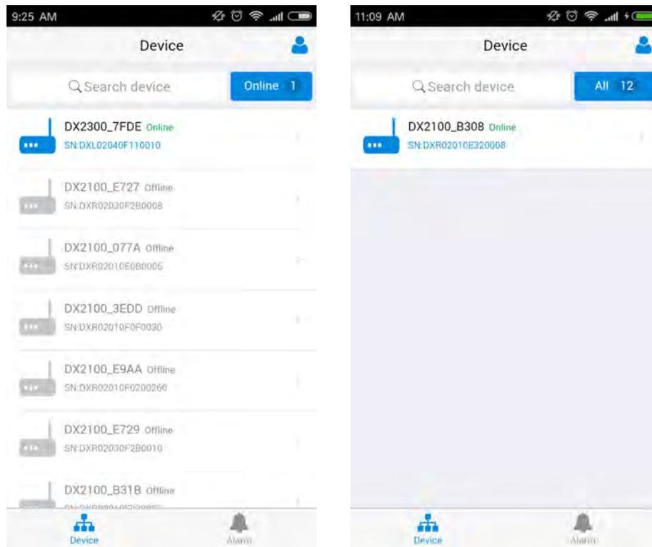
Device tab and alarm tab will be shown in the APP. In the device tab, the device information will be shown, including the value of registers of the remote device. And the value of the register can be changed in the APP as well. In the alarm tab, users can read the alarm messages.
