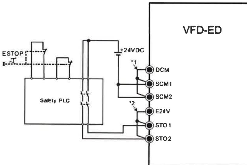
Figure 2, Possible connections for STO
