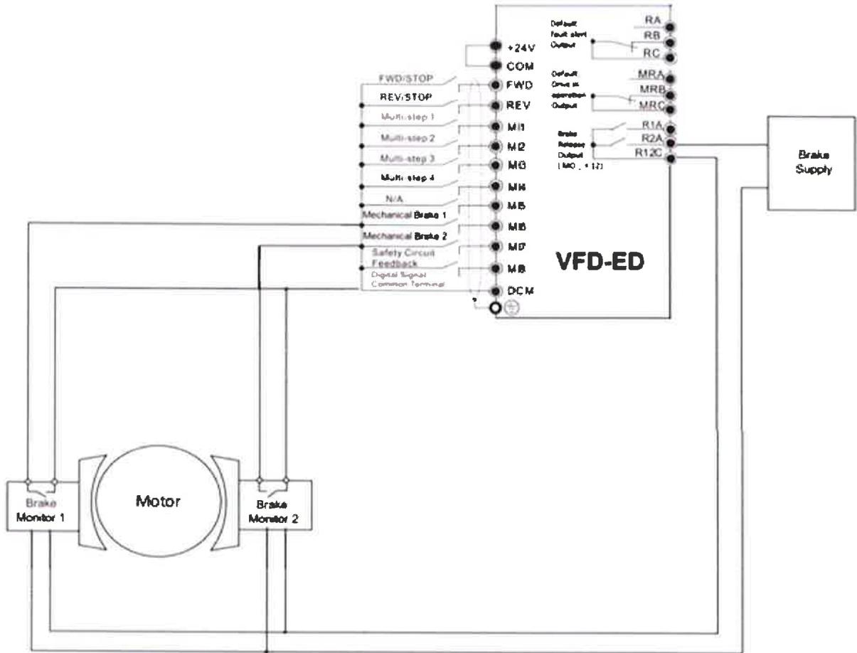
Figure 1, brake monitoring connections
