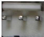
1 2 3 Figure 1.6 CN3 pin definition
