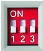
The dipswitches 1,2,3 are meant to be used in case there is no keypad.
