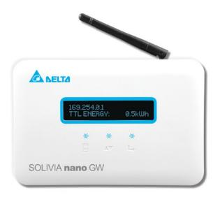
The SOLIVIA nano GW gateway is the communication interface for your micro inverters. It connects the nano 260 Micro Inverters in your PV system over the Internet to the SOLIVIA Monitor, Delta's monitoring system. You can then access important data for your solar system online.
