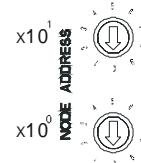
Example: If you need to set the node address of DVPDT02-H2 to 26, simply switch the corresponding switch of  $x10^1$  to 2 and the corresponding switch of  $x10^0$  to 6.
